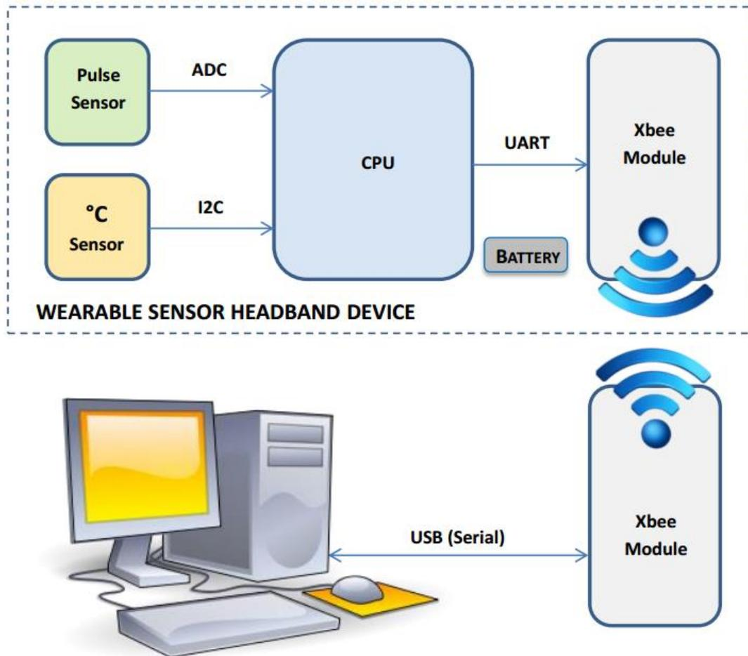
Fig.1. Principal representation of the wearable headband device work.
