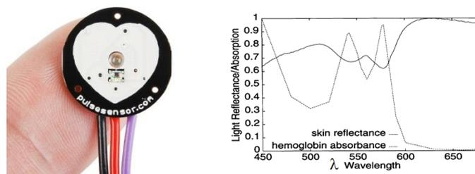
Fig .2. General view of the pulse wave optical sensor (left) and the relevant ratio of skin reflectance vs hemoglobin absorption according to  $\lambda$  (right).
