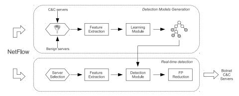
Figure 1: The system architecture of Disclosure. In the training phase (upper half), labeled training samples are used to build detection models. In the detection phase (lower half), the detection models are used to classify IP addresses as benign or associated with C&C communications.
