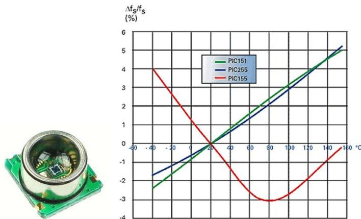
Fig .3. General view of the temperature sensor (left) and the temperature dependence of the resonant frequency  $\Delta f_s$  and the longitudinal oscillation  $f_s$  for three popular piezoceramic materials (right)
