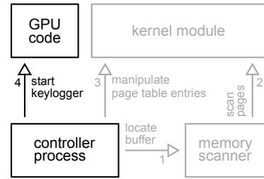
**Figure 1: Temporary and permanent components of the keylogger. Gray denotes bootstrapping operations, while black denotes monitoring functions.**
