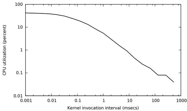
**Figure 4: CPU utilization of the keylogger for different GPU kernel invocation intervals.**
