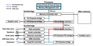
DMA attacks aiming at I/O controllers' internal memory:
