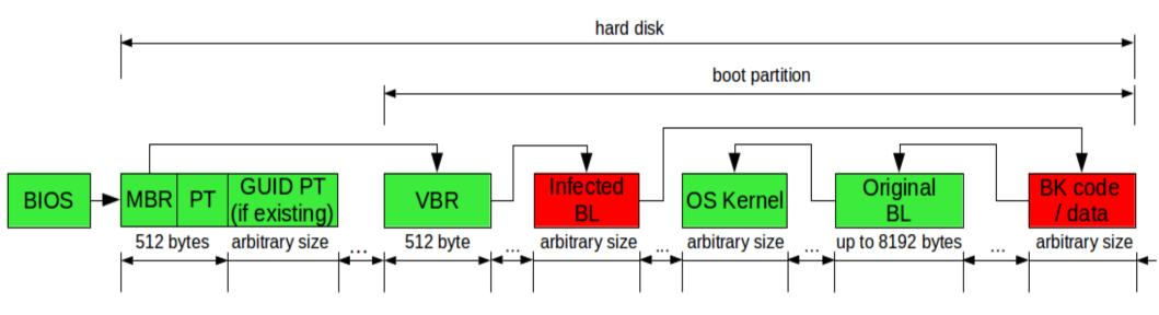
boot process with infected bootloader (BL)
